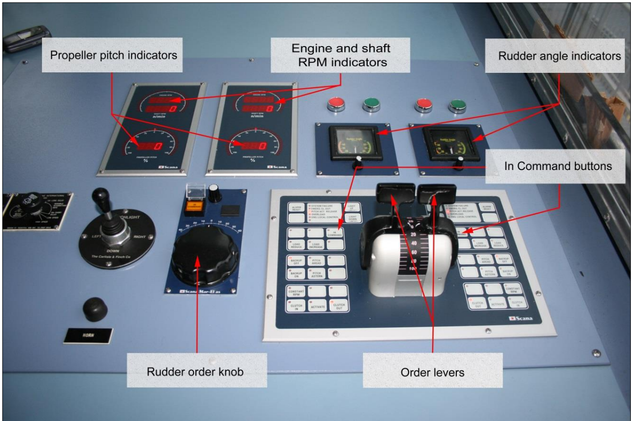
Figure 12. Photo of bridge control panel showing order levers, pushbutton controls and alarm displays, and engine and propulsion controls and indicators.
