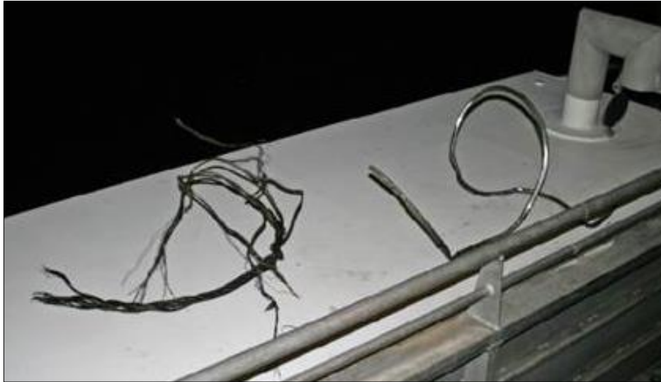
Figure 6. Debris found in ferry propeller, a 3-foot length of wire cable and 4-foot steel bar, both about half an inch in diameter.
