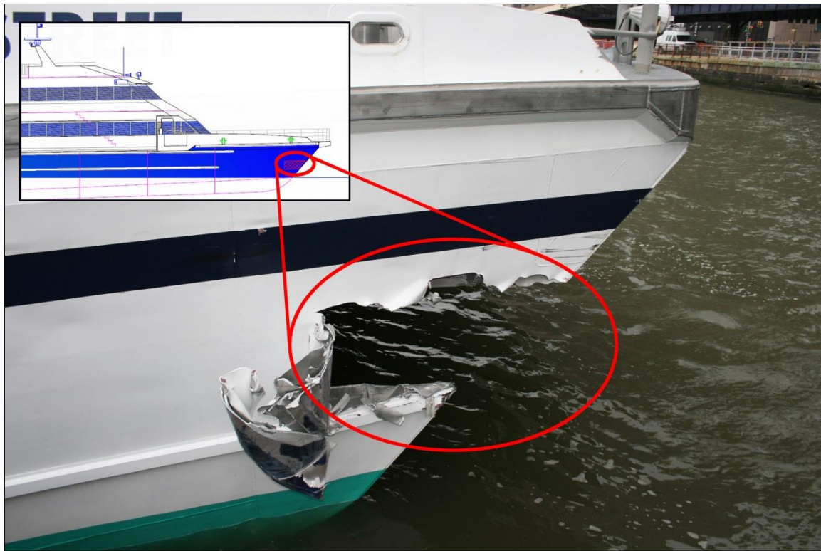
Figure 5. Damage to the Seastreak Wall Street starboard bow.
