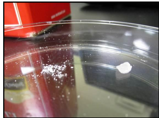
Fig. 6: Ice Cream Salt Control Sample After Crushing
