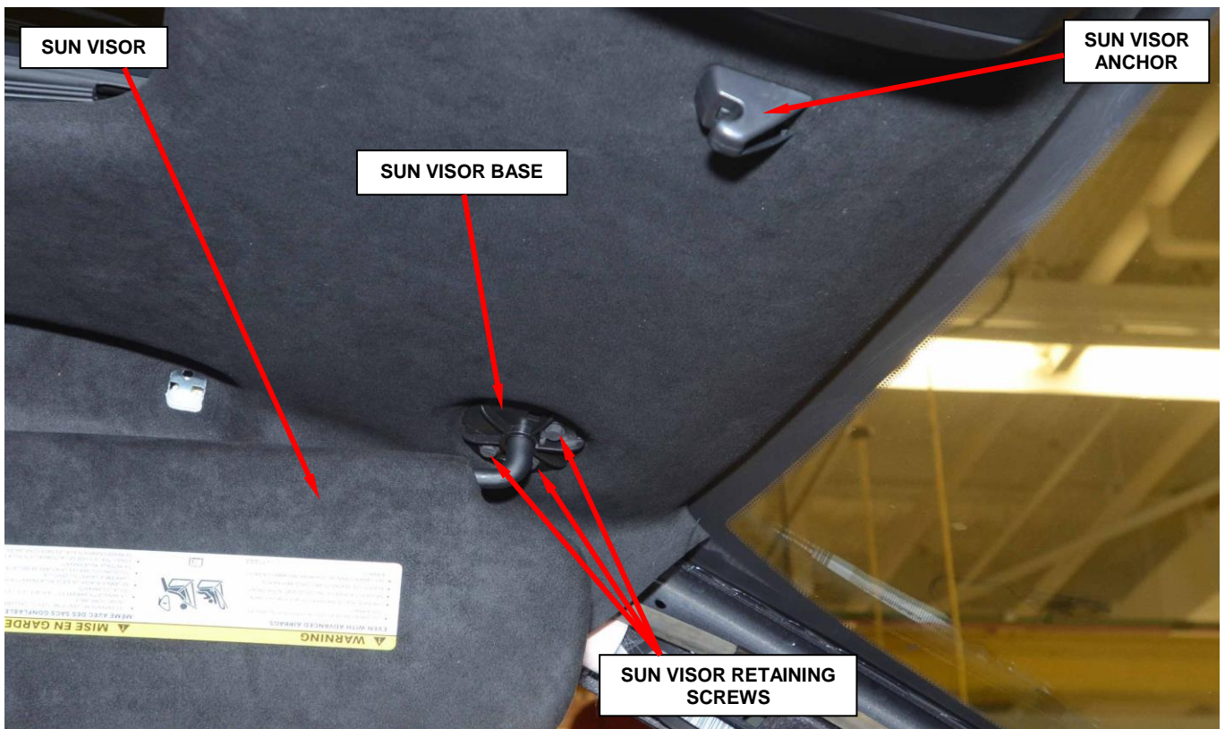
Figure 8 – Sun Visor Retaining Screws and Anchor
