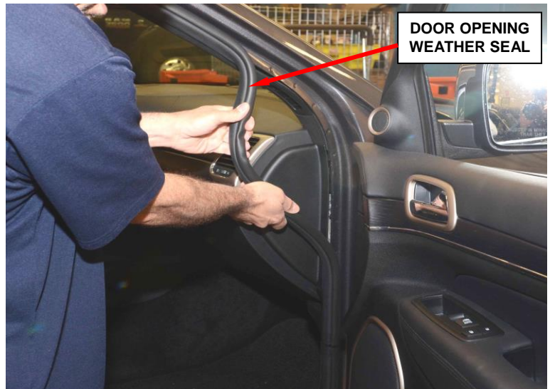
Figure 1 – Door Opening Weather Seal
