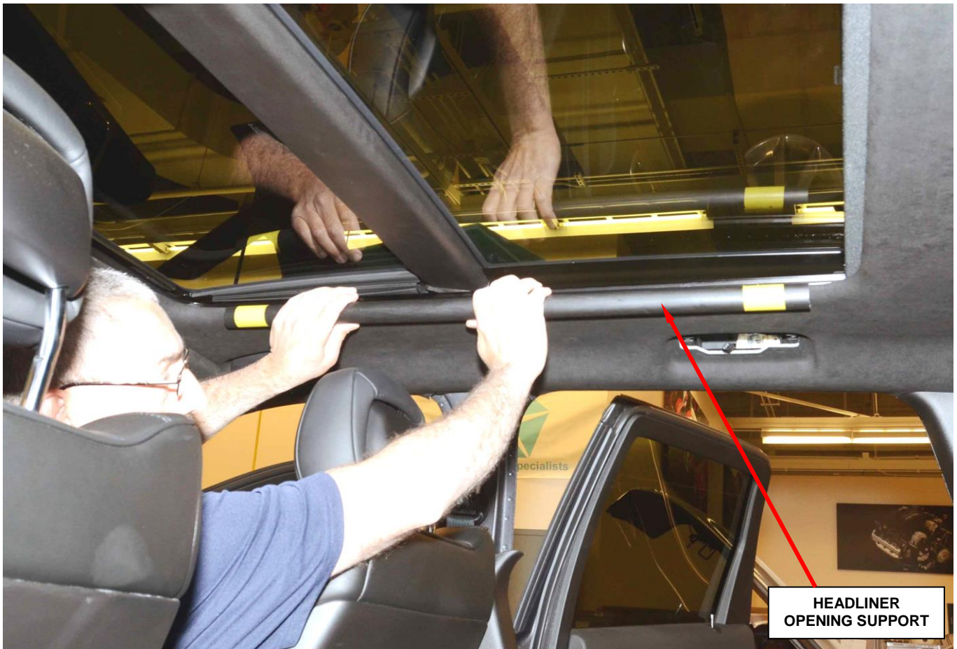
Figure 7 – Headliner Stiffener Tubes (Dual Pane Sunroof Only)
