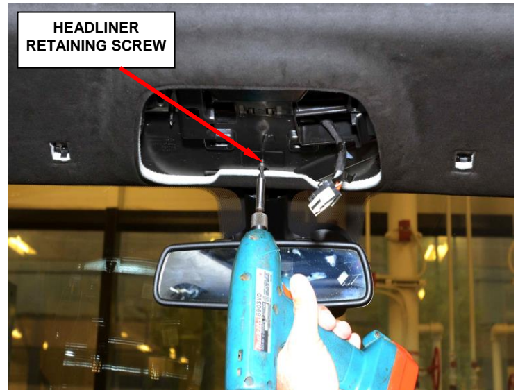
Figure 10 – Headliner Retaining Screw
