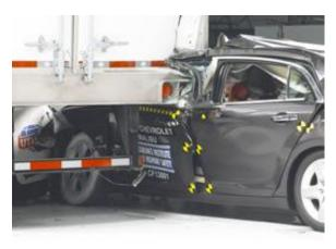
driver seat indicated serious injuries were unlikely. Similarly, in the underride tests in which the guards held up, the Malibu's structure and airbags protected the dummy, and injury measures were generally low and not life-threatening. In contrast, when the guards failed, head and neck injury measures were so high that real drivers would have died.
