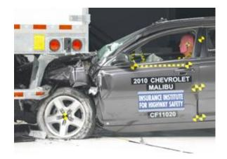
The underride guard on the Manac trailer, above, was the only one of eight tested to prevent underride in a 30 percent overlap crash. The performance of the Utility trailer, below, was more typical.
