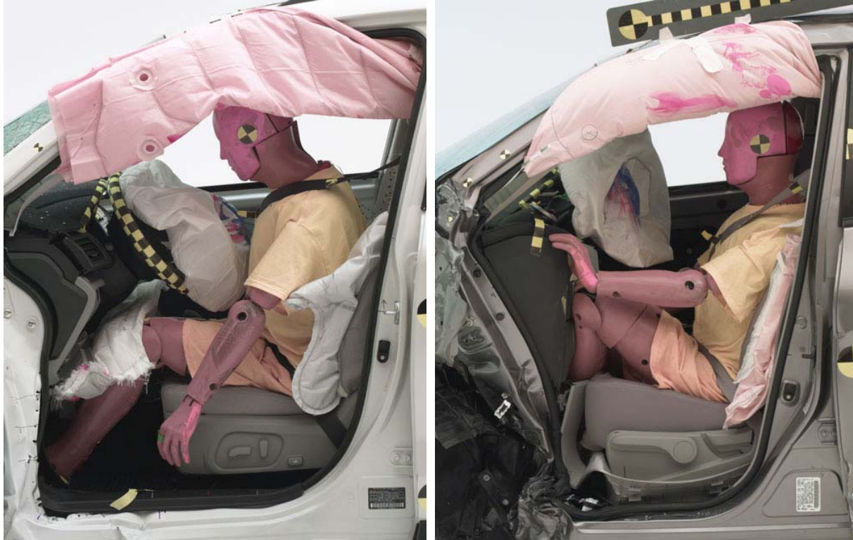
The structure of the 2014 Subaru Forester, left, held up well in the small overlap front test. The 2012 Nissan Rogue's poor structural performance was more typical of the small SUVs tested.
