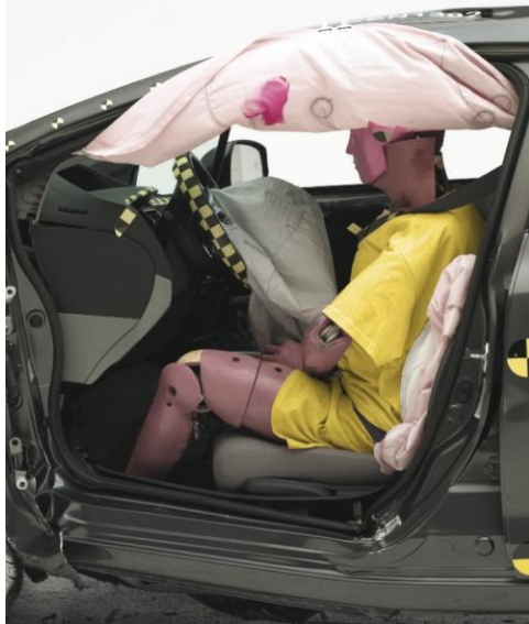
Significant occupant compartment intrusion contributed to the poor rating for the Nissan Sentra (top). The front wheel and tire were forced rearward in the test. In the 4-door Honda Civic (above) test, the occupant compartment stayed intact, preserving survival space for the dummy.
