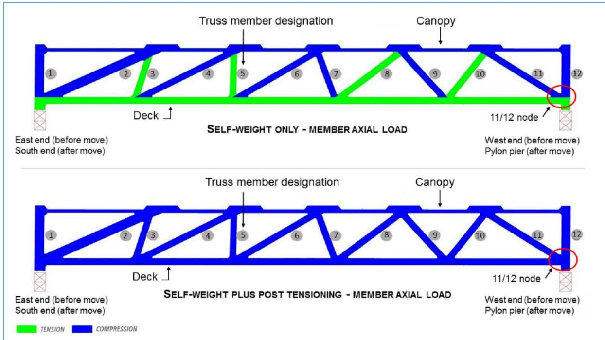
**Figure 21.** Self-weight axial forces only (top) for diagonal truss members 2 and 11, which are combined with post-tensioning forces concurrently acting on main span to produce net axial forces (bottom) at each end before transport and on permanent pier following transport. Top illustration is shown without post-tensioning; bottom illustration is shown with actual loads. (Source: FIGG, annotated by NTSB)
