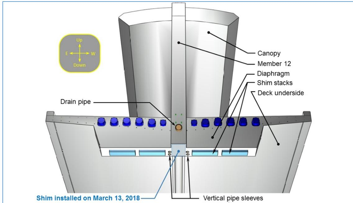
**Figure 23.** View of underside of post-SPMT support location of pylon diaphragm onto pylon pier, showing shim stacks on east and west side of diaphragm centerline. Post-SPMT support location is at underside of pylon pier deck. (Source: FHWA 2019)
