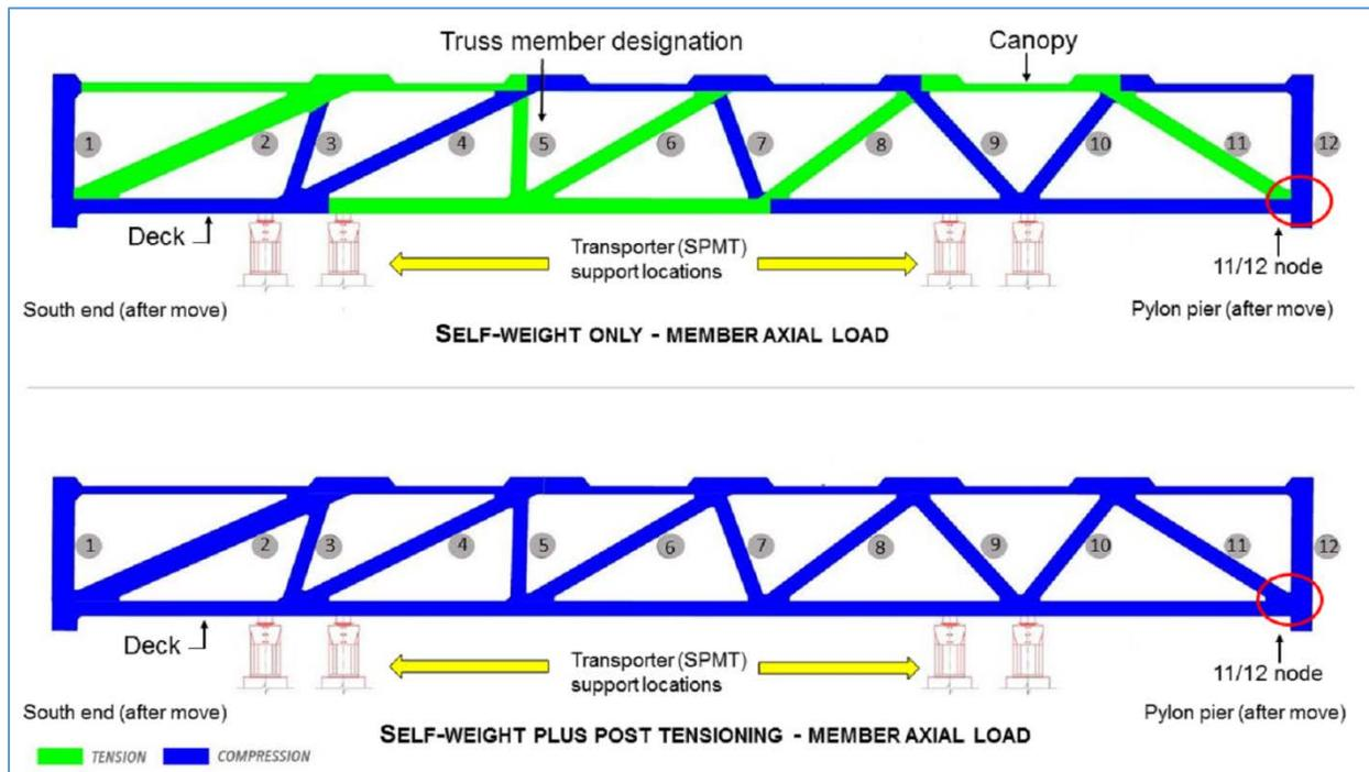
**Figure 20.** Main span tension and compression members for diagonal truss members 2 and 11, which supported each end during SPMT move from casting yard to south and pylon piers. Top illustration is shown without post-tensioning; bottom illustration is shown with actual loads. (Source: FIGG, annotated by NTSB)
