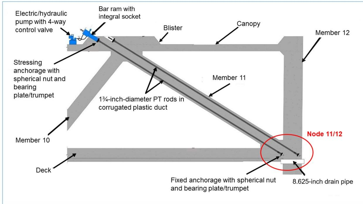
**Figure 19.** Main span, north end, showing post-tensioning specialized equipment in relation to location of PT rods in member 11. (Source: Structural Technologies, annotated by NTSB)
