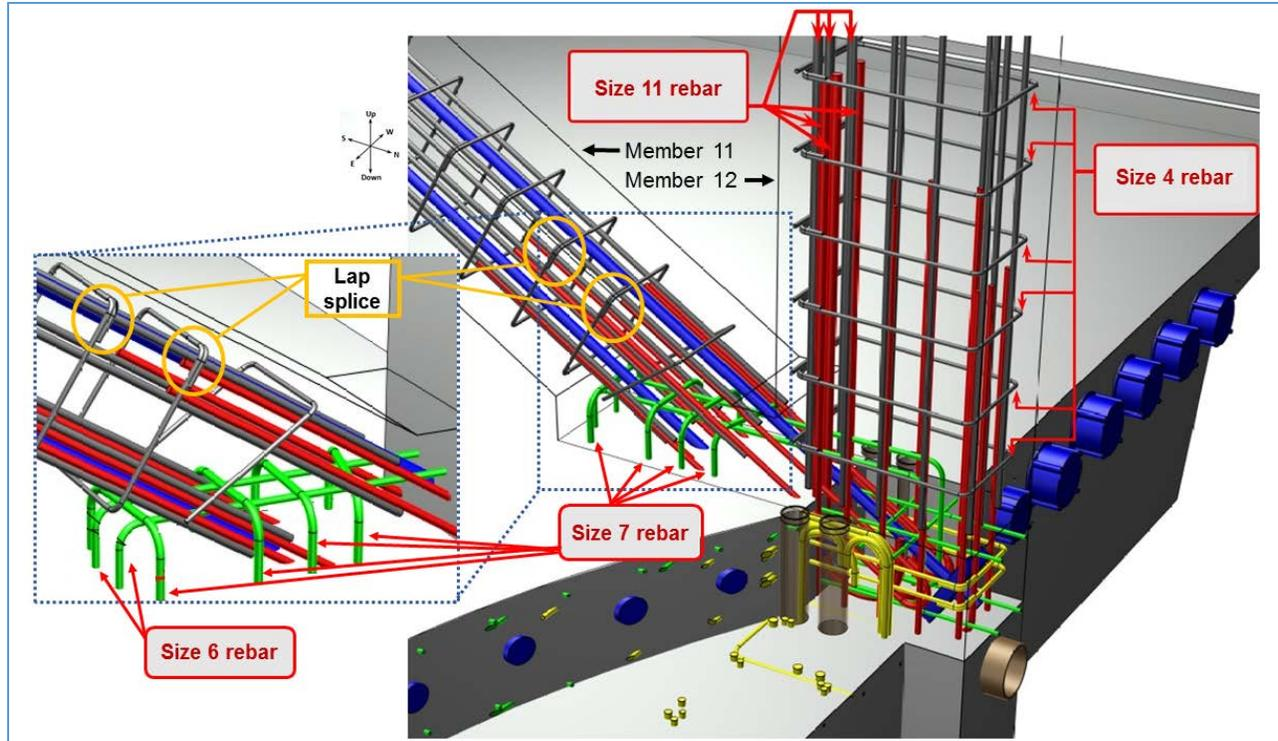
**Figure 17.** Main span, north end, showing rebar detailing in member 11, member 12, and node 11/12. Inset shows another view of rebar in node 11/12 and detail of lap splice from member 11. (Source: FHWA 2019)
