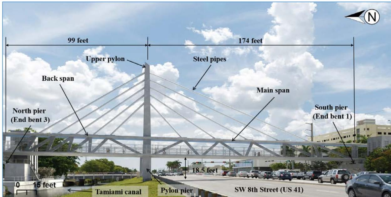
**Figure 2.** East-view rendering of completed UCPP pedestrian bridge. Note: This depiction does not illustrate the 11-foot northward shift of the bridge to accommodate a future westbound express bus lane on SW 8th Street or the construction of a bulkhead wall on the south Tamiami Canal bank. (Source: FIU, annotated by NTSB)
