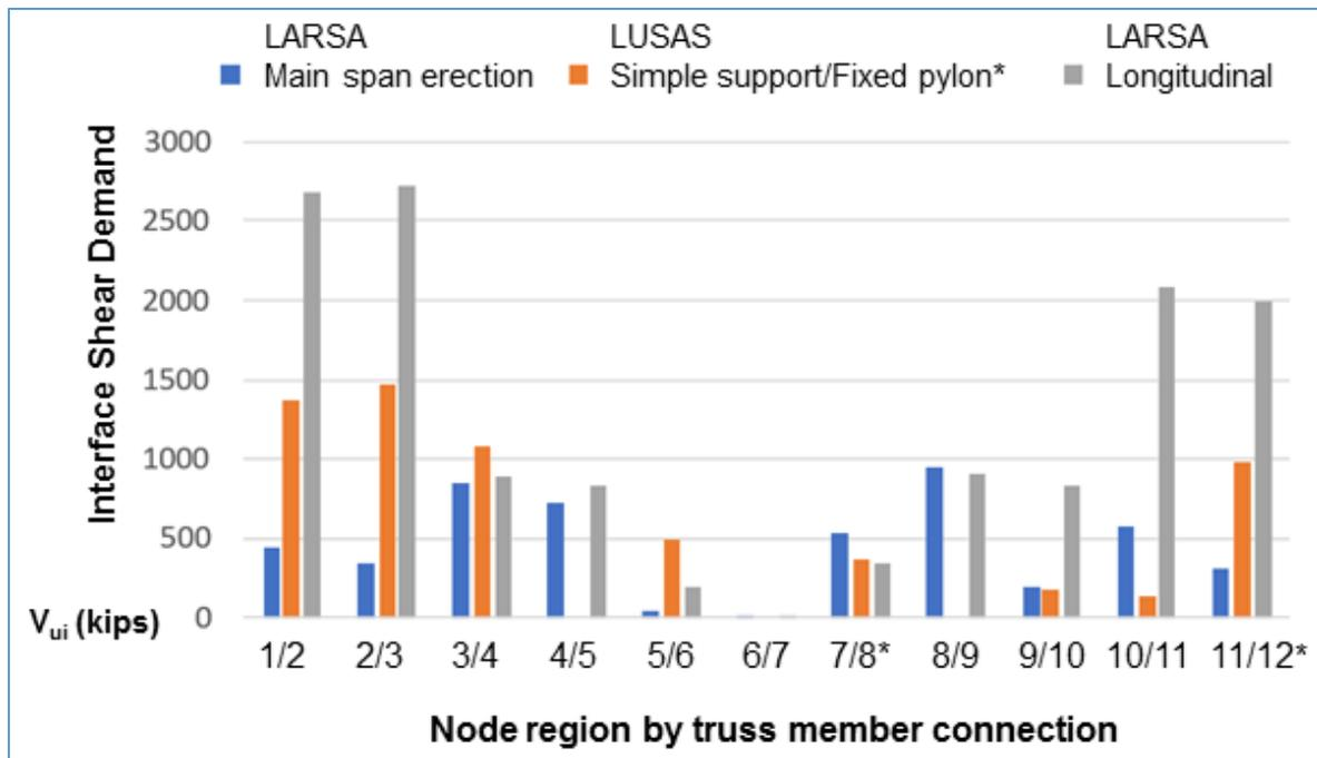
**Figure 27.** Nodal region interface shear demand results generated for FIGG bridge design, with horizontal axis showing two truss member identification numbers that connect into each nodal region. (Source: FHWA 2019)
