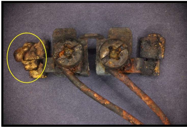
Figure 11 – Plug blade with localized melting
